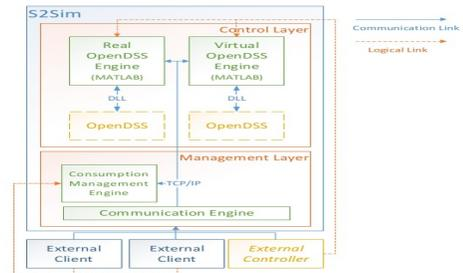
Figure 1. The communication structure in  $S^2$ Sim
