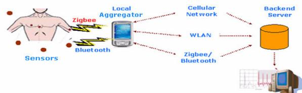
Figure 1: Wireless healthcare system architecture
