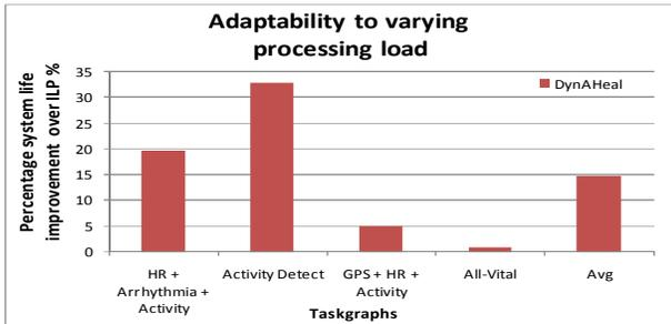
Figure 3: System life improvement achieved by *DynAHeal* over ILP when task execution times change at run-time
